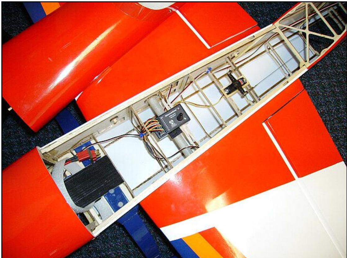
**Figure 5 – XtremeLink™ 8 channel receiver installation**
