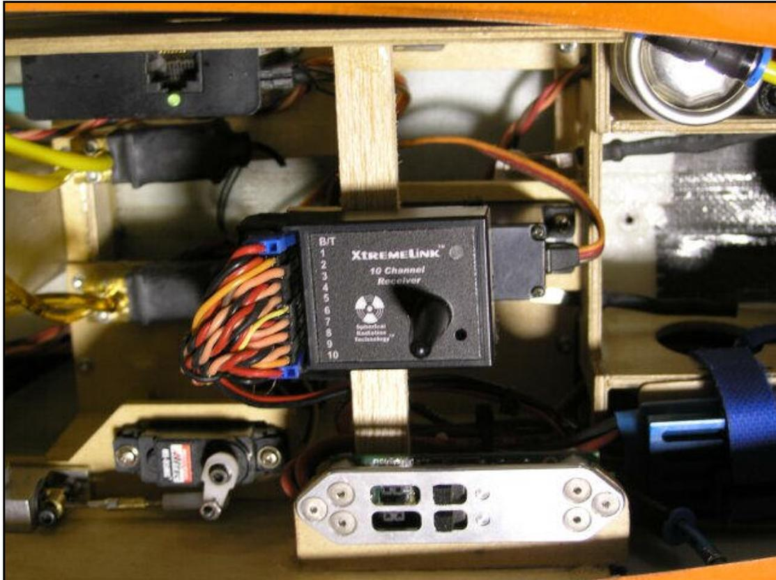
**Figure 6 – XtremeLink™ 10 channel receiver installation**
