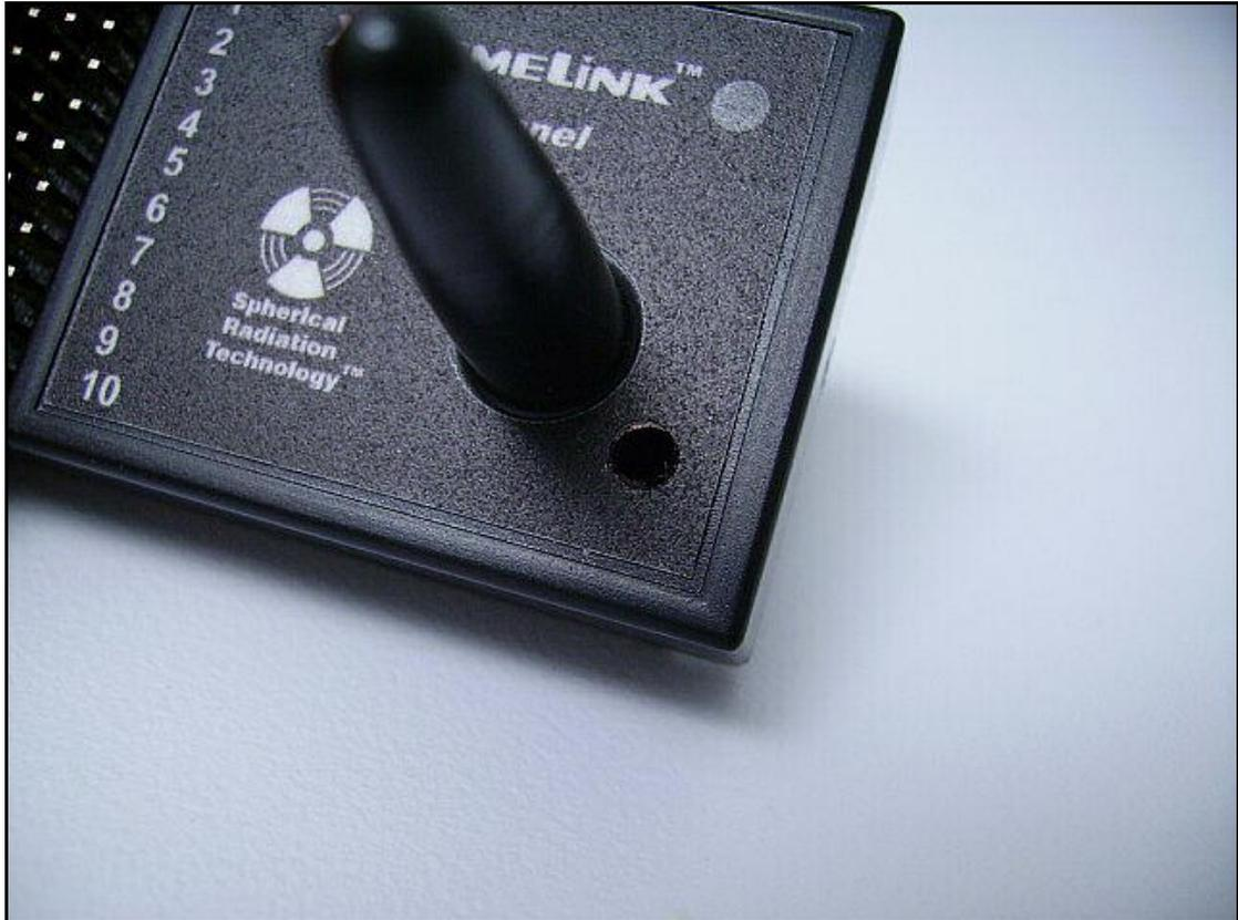
**Figure 7 – XtremeLink™ receiver programming button location**
