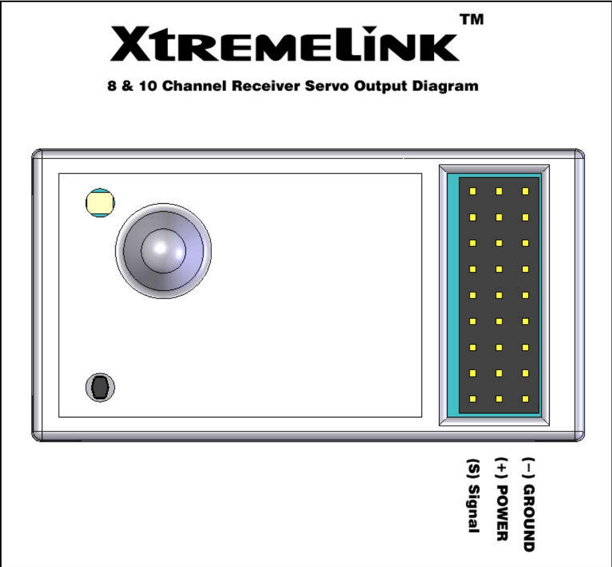
**Figure 8 – XtremeLink™ receiver servo output polarity**
