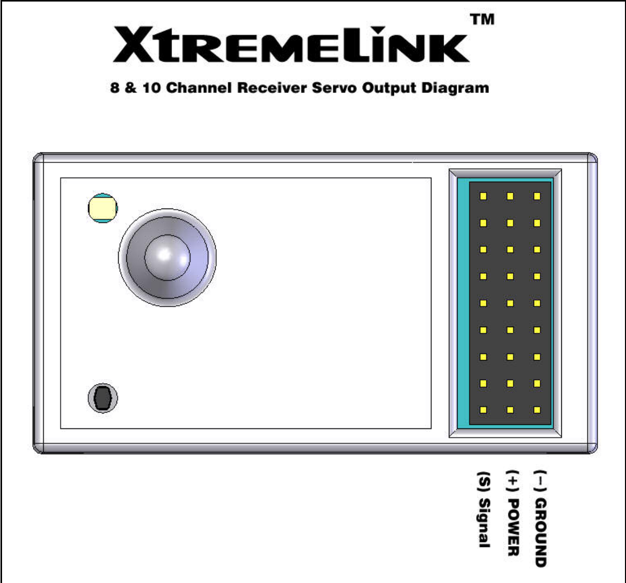
Figure 8 – XtremeLink™ receiver servo output polarity
