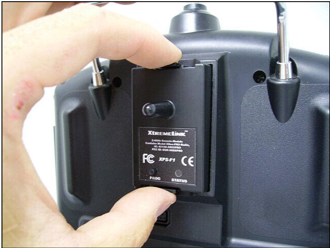
Figure 3 – Futaba XtremeLink™ module installation
