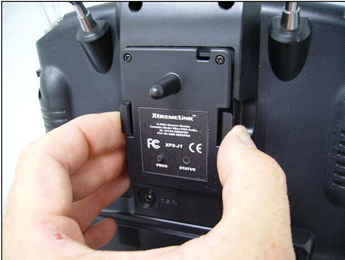
Figure 4 – JR XtremeLink™ module installation
