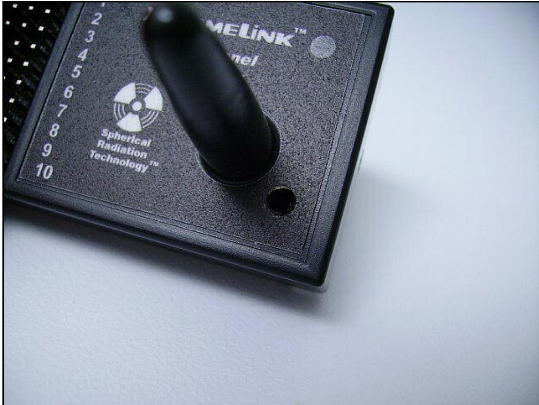
Figure 7 – XtremeLink™ receiver programming button location
