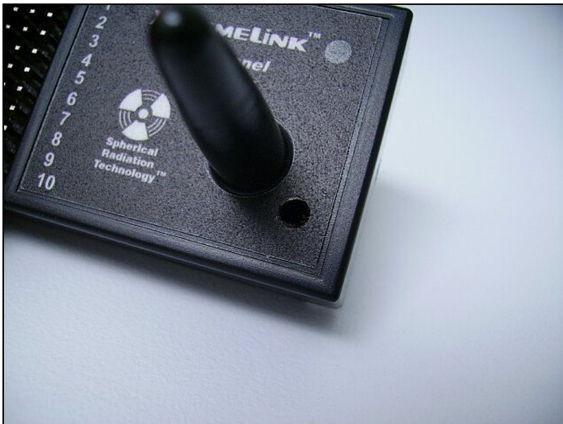
Figure 7 – XtremeLink® receiver programming button location
