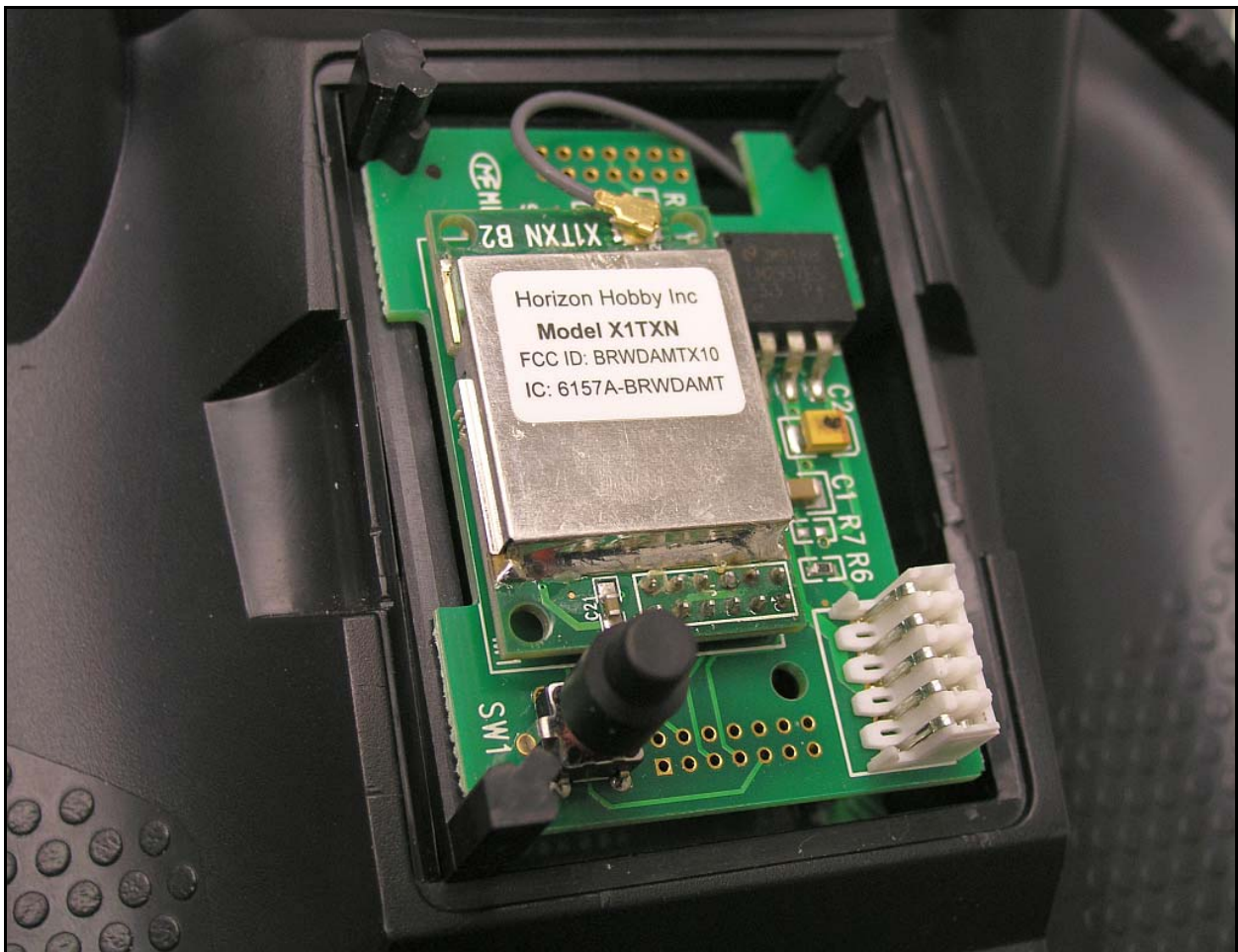
Figure 2 – Pull up to unplug stock RF module board
