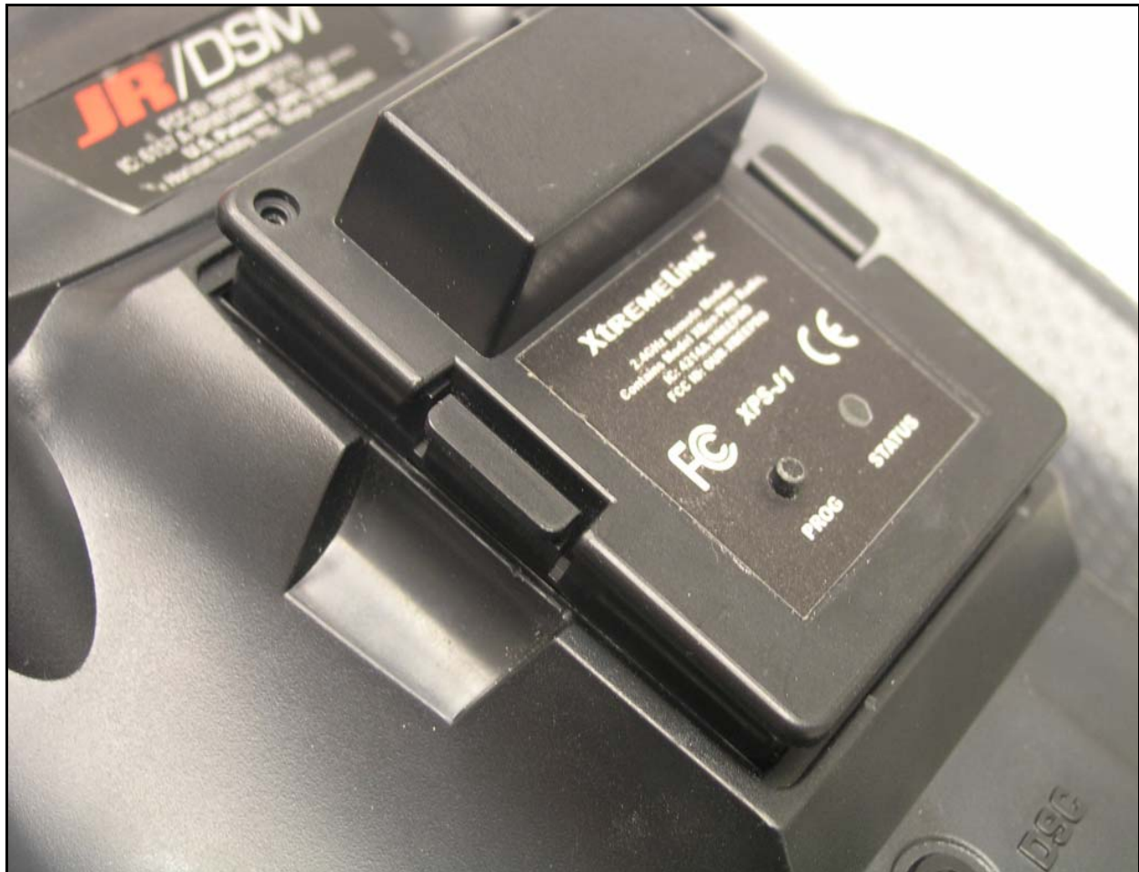
Figure 11 – Set module assembly in place
