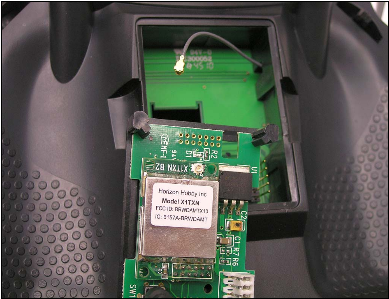
Figure 4 – Remove RF board assembly
