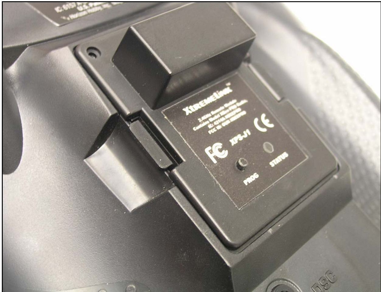
Figure 12 – Module fully seated
