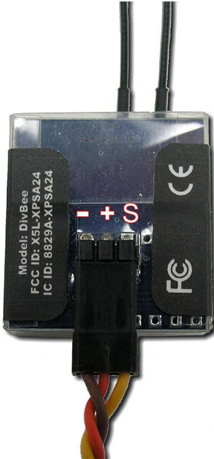
Figure 1 – RFU plug polarity details
